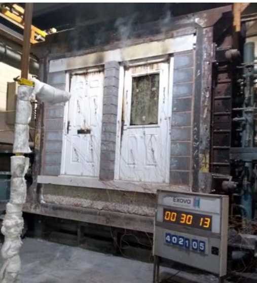
7mm Pyrodur with 6.8mm Clear
